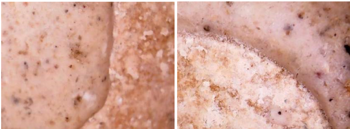
Figure 10. Interface of the two components. The union of a selected putty plate with a rock presents a homogeneous union without separations, after the exposure of the accelerated aging chamber
