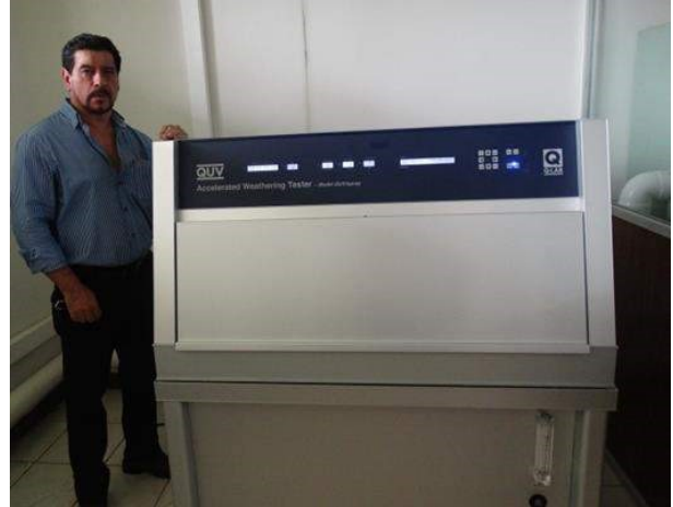
Figure 8. Accelerated aging chamber used in the test
