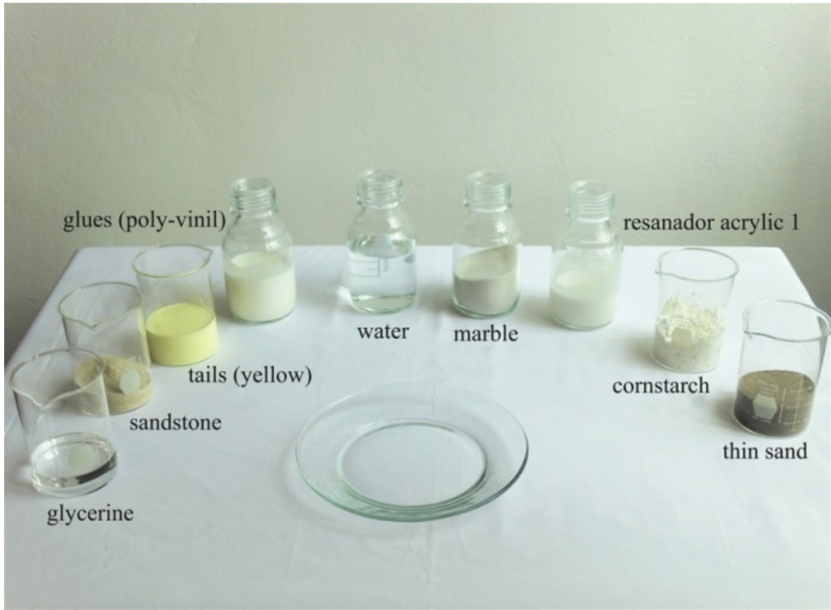
Figure 1. Main components used in the elaboration of the sandstone finishing mass
