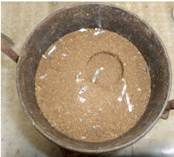
Figure 11. CBR test - reinforced soil
