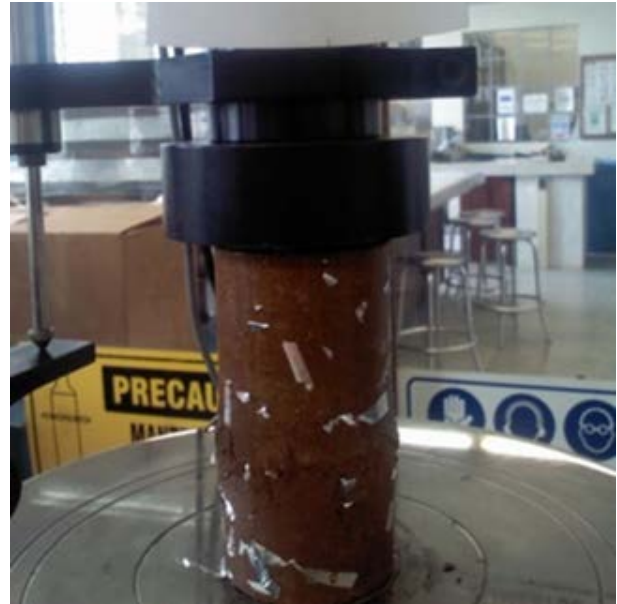
Figure 8. Reinforced soil cylinder failures
