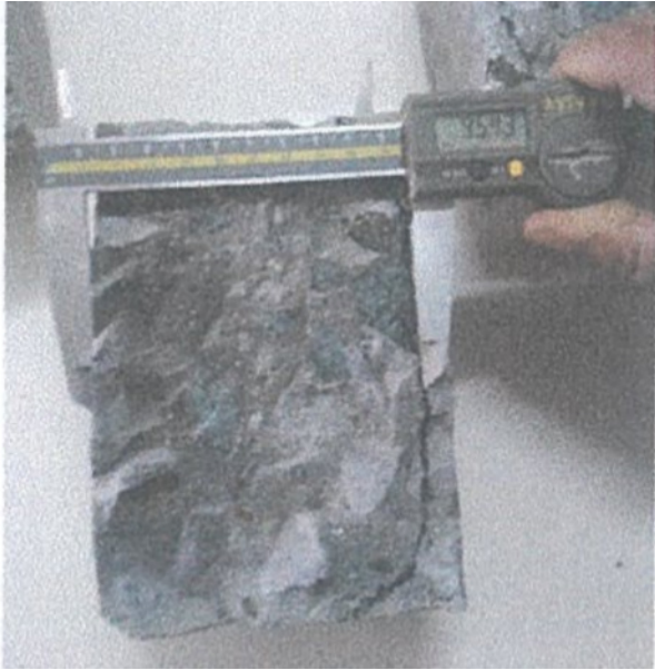
Figure 3. Measurement of water penetration depth by using a caliper
