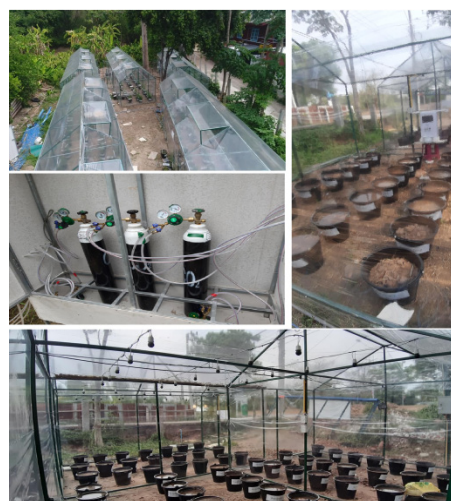
Figure 1. Open Top Chamber for field studies of elevated air temperature and CO 2 concentration on rice
