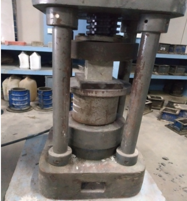
Figure 1. Test for Compressive Strength of ECC mixes.
