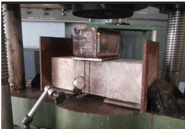
Figure 10. Shear Bond Strength Specimen Set Up
