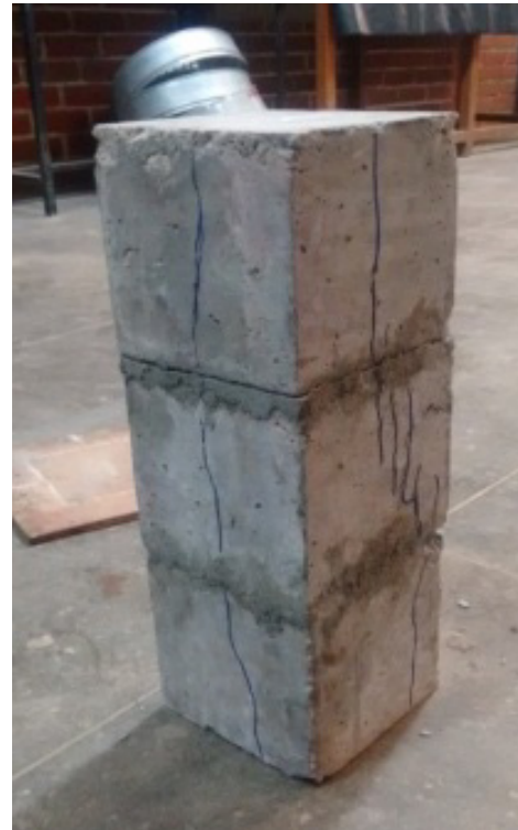
Figure 7. Masonry prism set up for Compression Test
