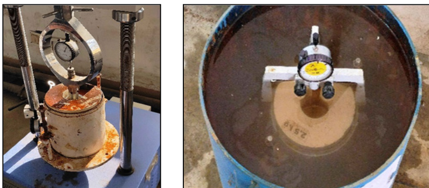
Figure 3. Experimental setup for soaked CBR Test
