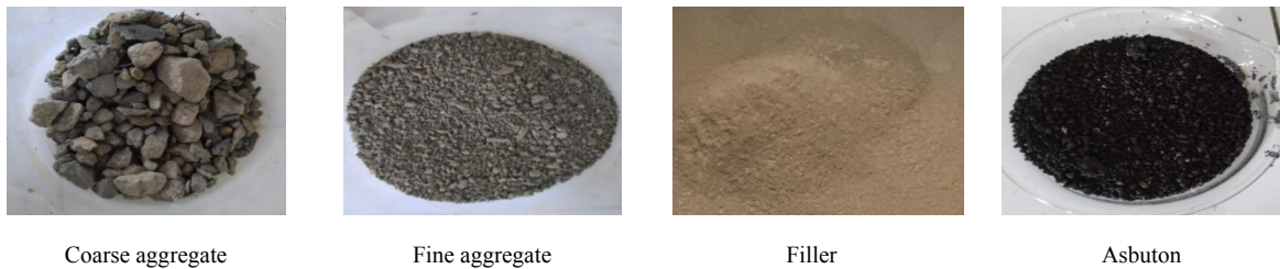
Figure 3. Coarse aggregate, fine aggregate, filler and Asbuton
