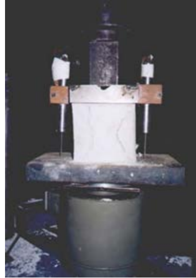
Figure 5. Compression test layout of mortar
