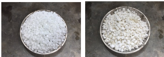
Figure 1. (Left) Expanded polystyrene foam aggregate (EPS) and (Right) Modified recycled expanded polystyrene foam aggregate (MEPS).
