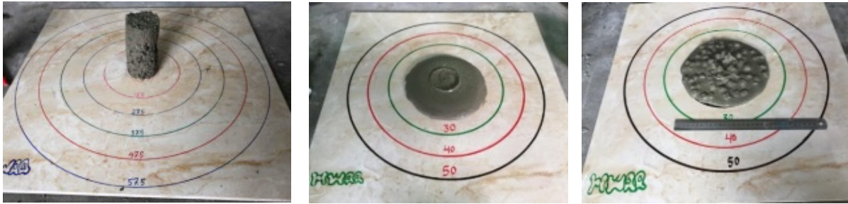
Figure 3. Flowability of (left) normal concrete (NC) (middle) foamed concrete (FC12) and (right) with polystyrene aggregate (FCE15)
