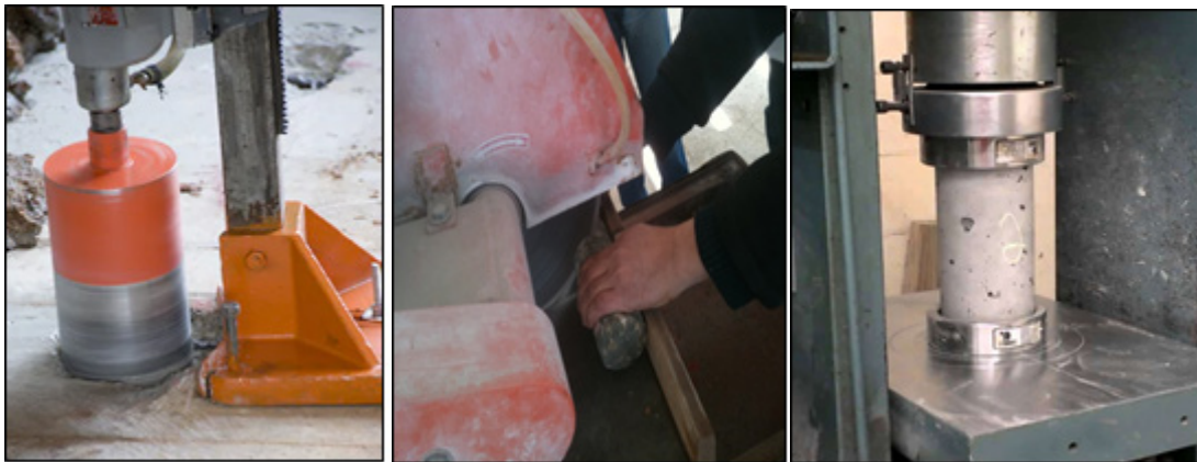
Figure 7. Core preparation. (a) Taking a core sample from a concrete block; (b): Preparation of the ends of the concrete core; (c): Compressive strength test of core sample.
