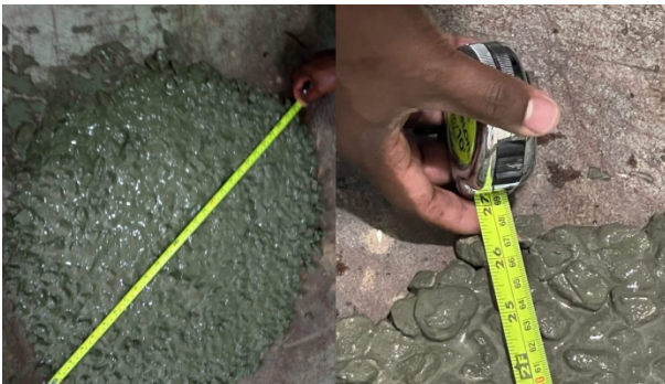
Figure 1. Calculation of SCGPC Slump value
