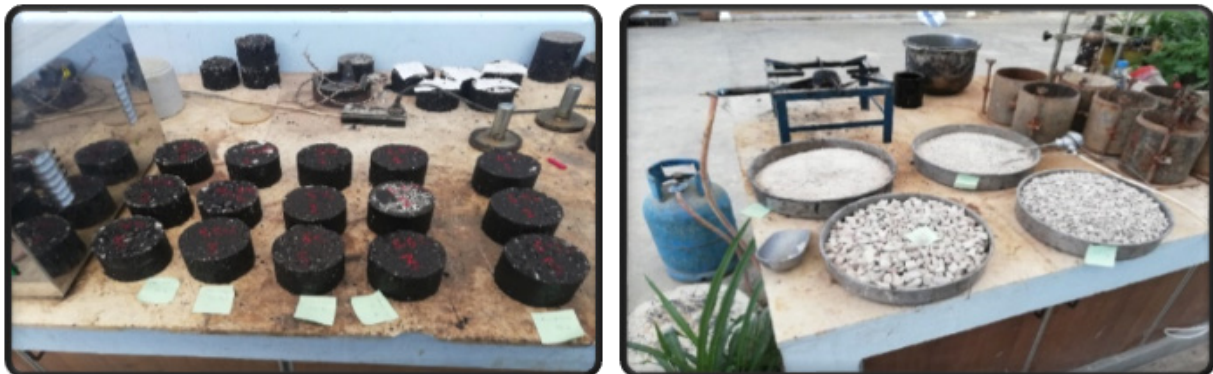
Figure 2. Creating asphalt mixtures according to the Marshall method
