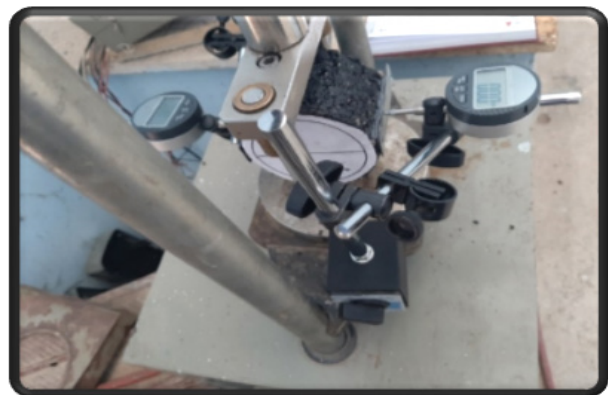
Figure 6. Preparation of asphalt samples for determination ITS
