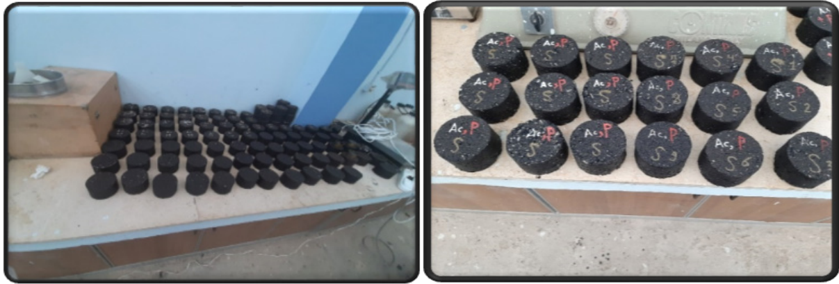
Figure 4. Some asphalt samples that were formed to study changes in the properties of asphalt mixtures
