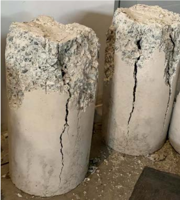
Figure 4. Control Specimen Splitting Failure Mode
