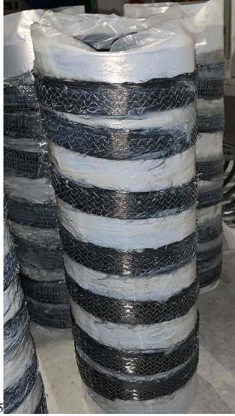
Figure 3. Finished Spiral on PVC Pipe Mold
