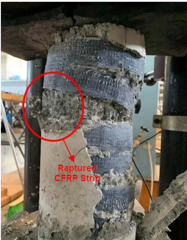
Figure 5. CFRP Spiral Specimen Failure Raptured CFRP Spiral Strip
