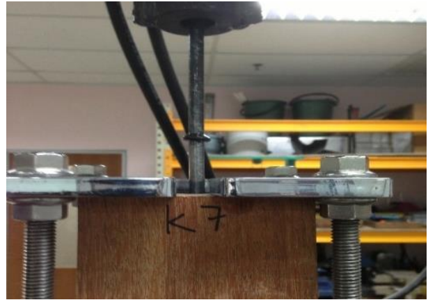
Figure 24. Specimen Failure in Rod-Adhesive
