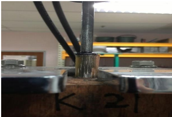
Figure 22. Pull-out Timber Failure after Test
