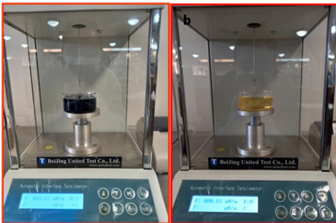
Figure 1. Tension determination with a platinum ring
