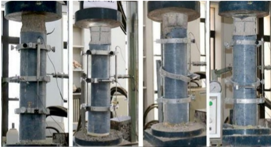
Figure 1. Setup for a test of SCC BFRP columns
