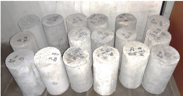
Figure 5. The specimens of concrete and RTC mortar strength test
