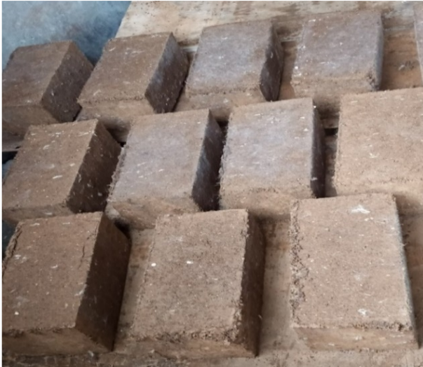
Figure 5. Bricks under curing
