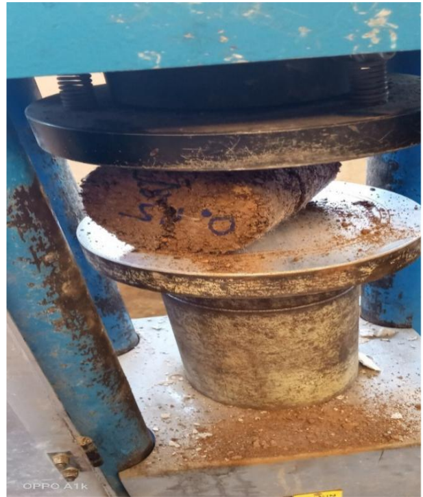
Figure 6. Splitting tensile test
