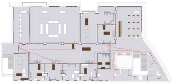
Figure 12. Evacuation routes on the second floor
