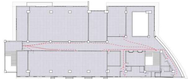
Figure 13. Evacuation routes on the third floor
