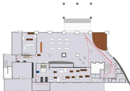
Figure 10. Evacuation routes on the ground floor
