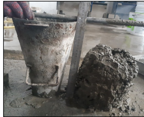
Figure 3. Slump height testing procedure
