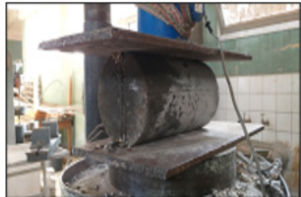
Figure 5. Test setup for Indirect tensile strength
