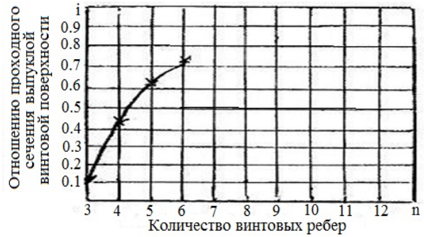
Figure 7. The dependence scheme of the area on the number of screw edges of the screw body
