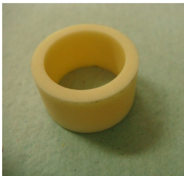
Figure 1. Alumina substrate (Al 2 O 3 ) used for electroless Ni plating
