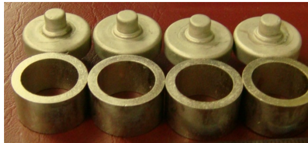
Figure 4. Electroless Nickel plating on tubes and buttons
