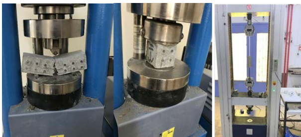
Figure 7. Setup of compression, flexural and pull out tests
