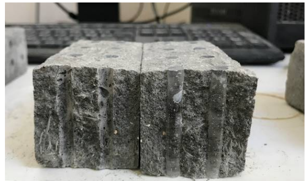
Figure 11. Cross-sections of flexural test specimens
