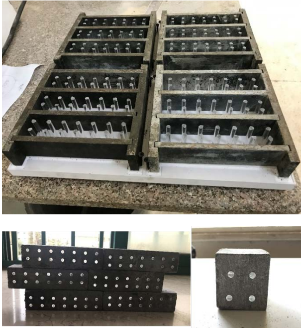
Figure 6. Specimens prepared for compression and flexural tests
