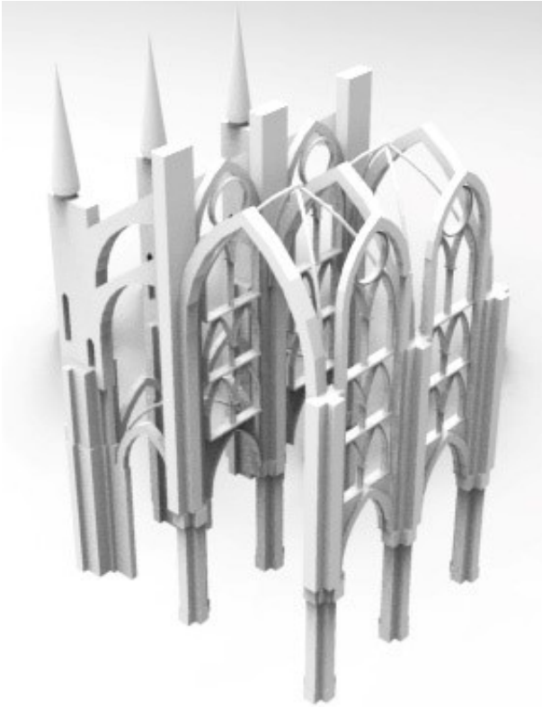
Figure 1. Central European Gothic structural form [5]
