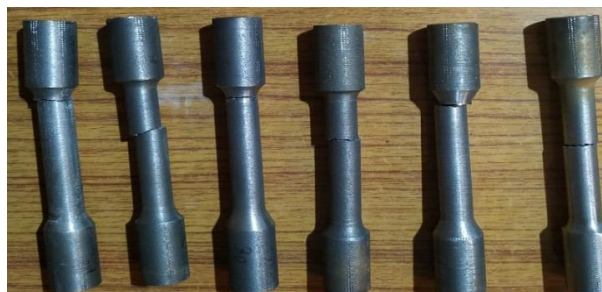
Figure 6. Tensile bar after tensile testing procedure
