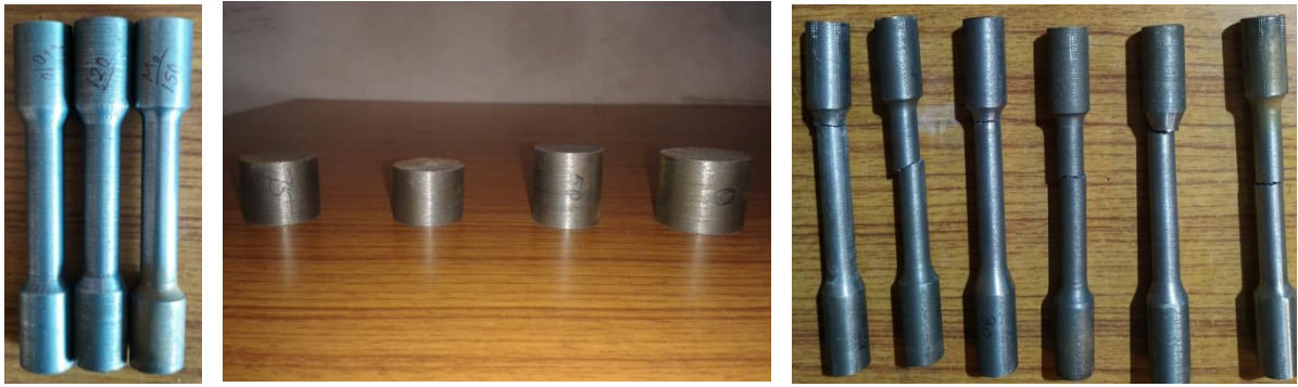
Figure 3. Systematic representation of break down tensile test bars and grinded test piece for hardness test
