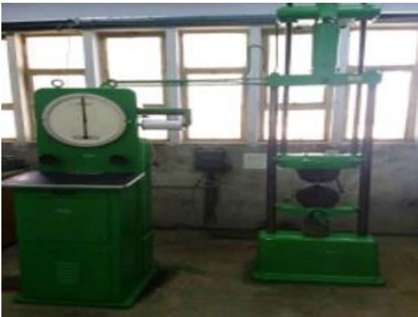
Figure 4. Universal tensile machine UTM used for mechanical tests on the specimens
