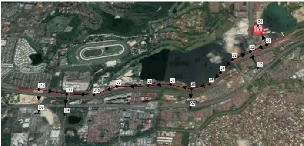
Figure 6. Sketch of the drainage network in the SWMM Model
