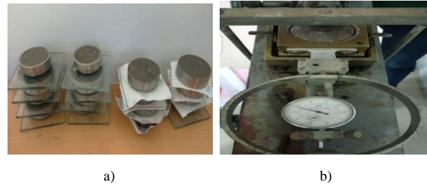
Figure 2. Sample fabrication process and shear resistance test Sample for shear resistance; b) Shear resistance test
