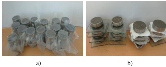
Figure 1. Sample fabrication process and conducting the test a) Test sample of compressive strength; b) Test of total strain modulus
