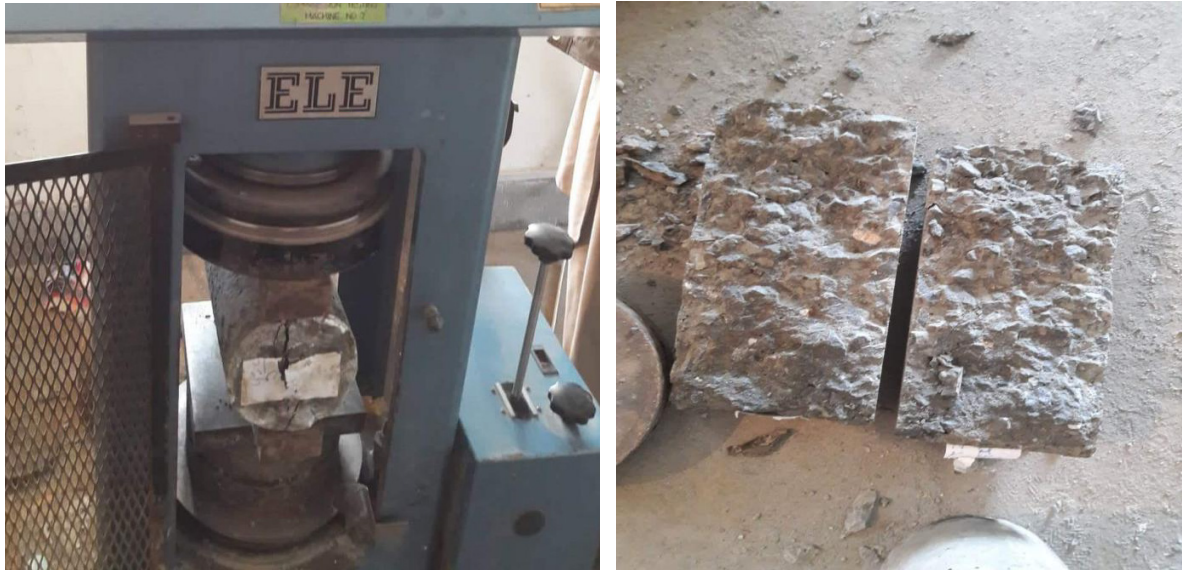
Figure 3. Setup for Split Tensile Strength
