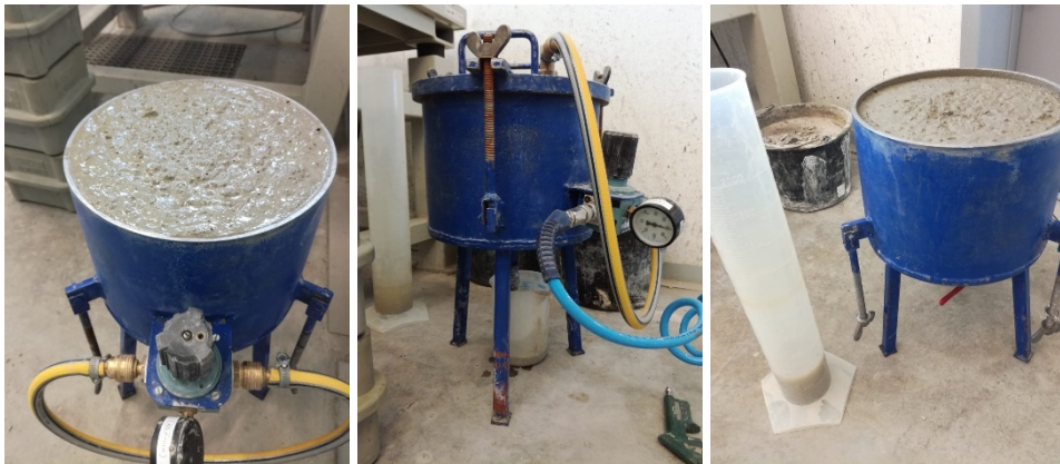
Figure 5. Equipment for determining water separation from concrete according to ÖBV during and after the test
