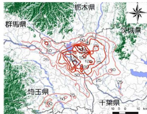
**Figure 8.** Subsidence based on leveling measurement from 1990-1994[6]
