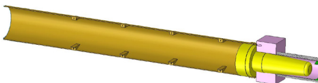
Figure 19. Representation of the final channel closure plug mounting
