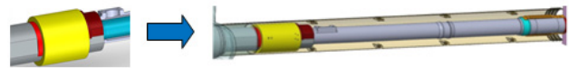
Figure 29. Representation of the device coupling steps and the protective cylindrical screen mounting
