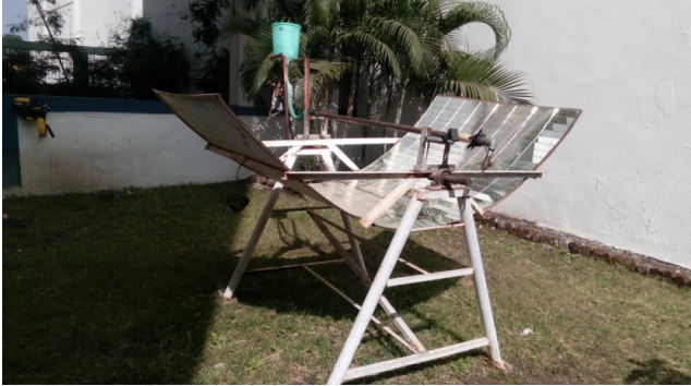
Figure 2. Fabricated parabolic solar collector with polished mirror collector
