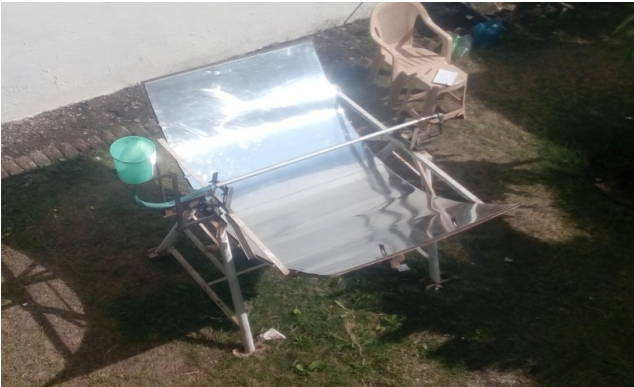
Figure 3. Fabricated parabolic solar collector with polished aluminium sheet collector
