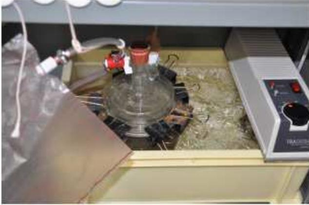
Figure 1. Batch Experiment with 2 L digester.
