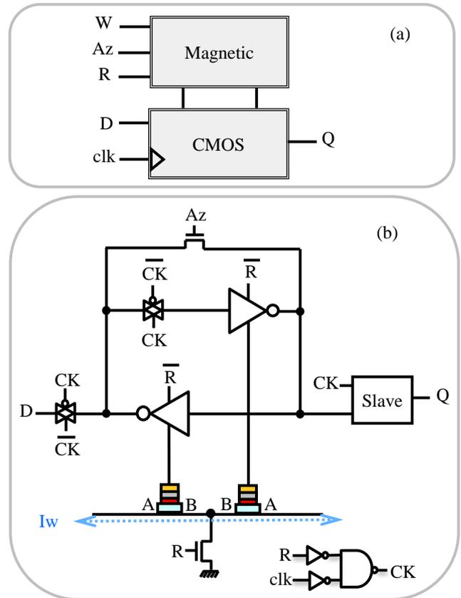
Figure 3. SOT based NVFF (a) Symbol of the NVFF with the corresponding inputs and outputs (b) Detailed architecture
