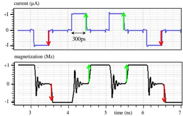
Figure 2. Validation of the SOT-MTJ Verilog-A compact model through electrical simulations
