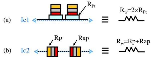
**Figure 5.** Equivalent resistance of the writing path (a) SOT device (b) STT device
