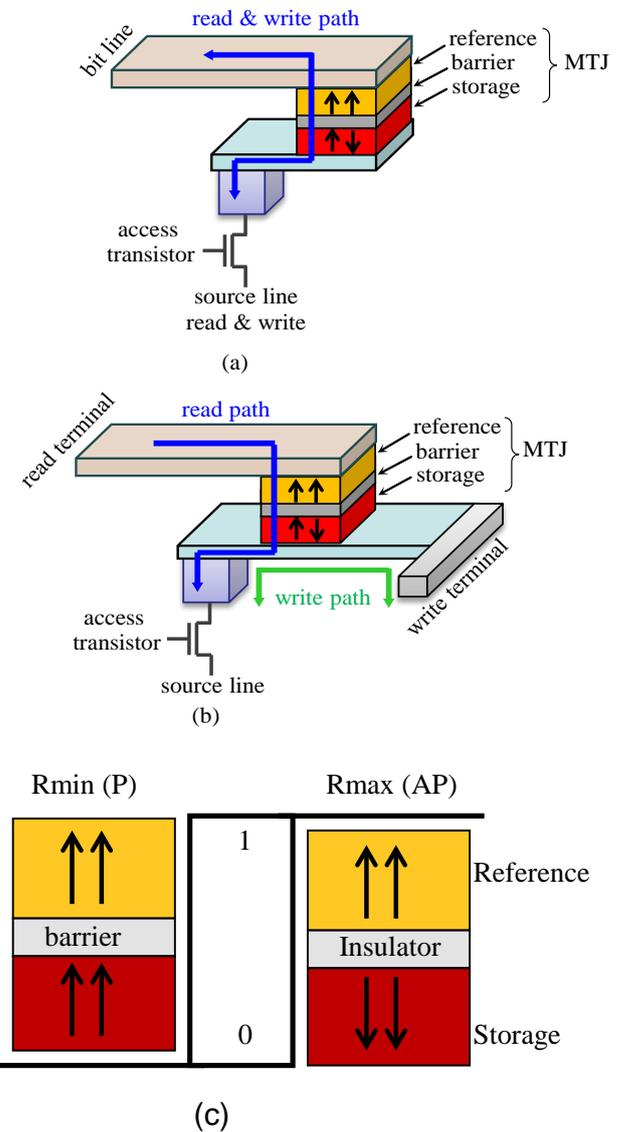
**Figure 1.** Comparison of MTJ based standard bit-cell (a) STT-MTJ based bit-cell (b) SOT-MTJ based bit-cell, In-plane current injection through the write line induces the perpendicular switching of the storage layer (up or down) (c) Resistance variation of the MTJ according to the storage layer magnetization state
