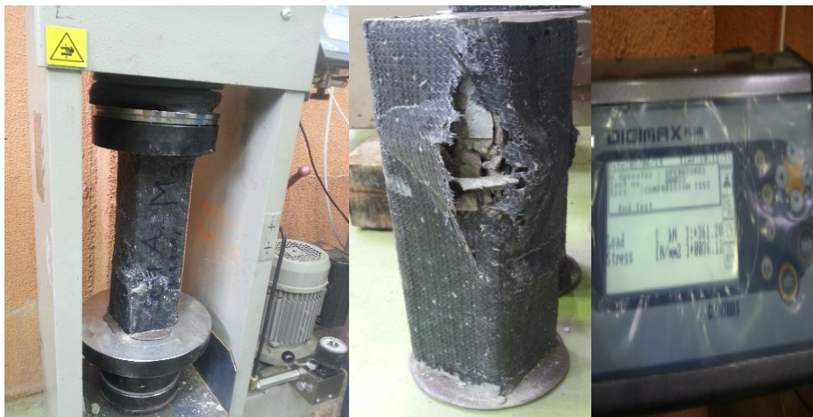
Figure 3. Test set up and shape of failure of rectangular (fully wrapped) specimens
