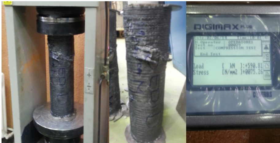
Figure 2. Test set up and shape of failure of circular specimens
