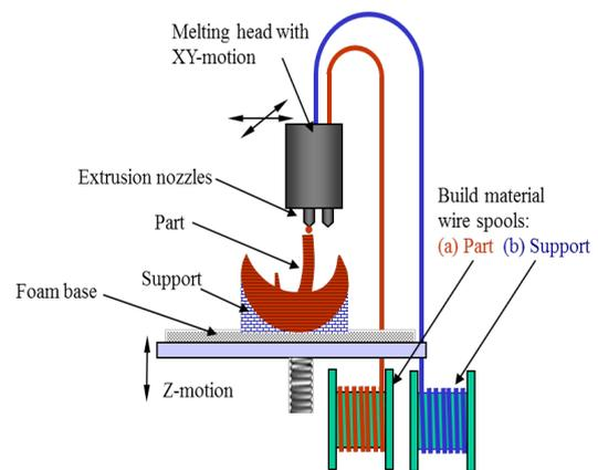
Figure 1. Schematic diagram of FDM [1]
