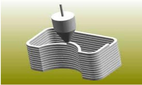
**Figure 2.** Layers visible on FDM part [2]
