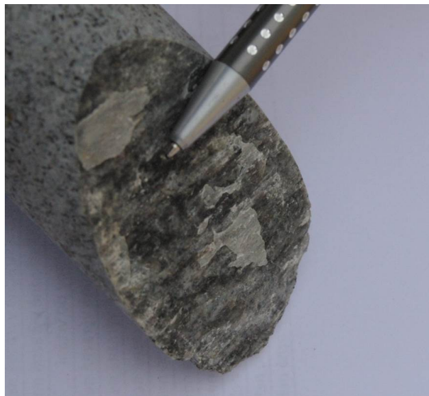
Figure 9. Kinematic indicators on the borehole core TIV_1.
