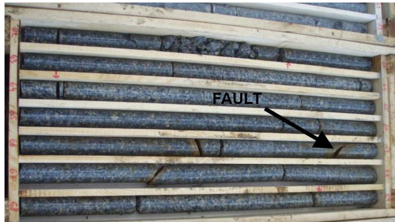
Figure 8. The core of borehole TIV_1. Fault plane is marked by arrow.
