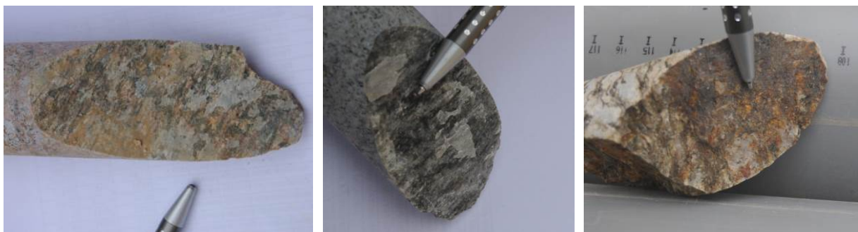
Figure 1. Kinematic indicators on granite core samples, striation (on the left), steps (in the middle) and groves (on the right).
