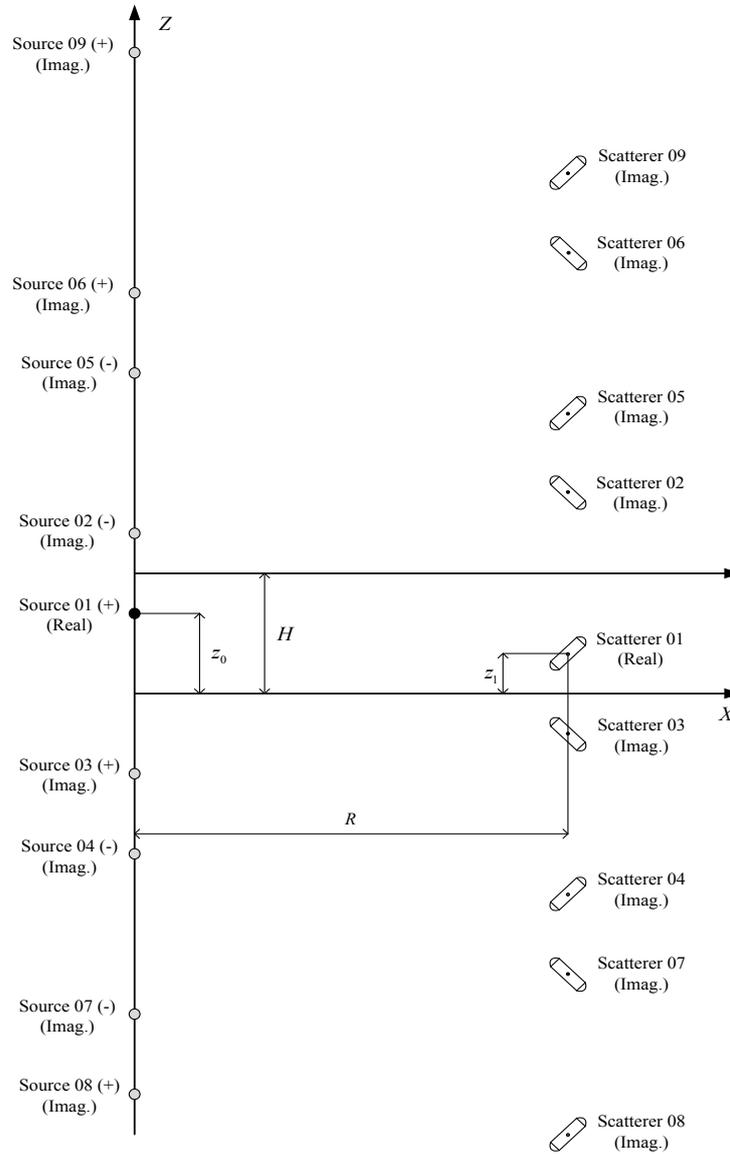
**Figure 1.** The mutual disposition of the impulse point-sources and scatterers in the plane waveguide
