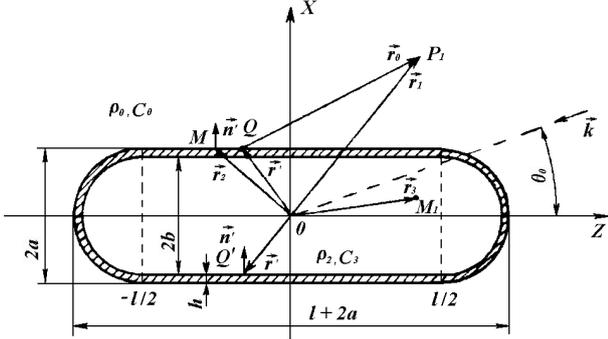
**Figure 2.** The elastic shell in the form of the terminal cylinder with the semi-spheres.
