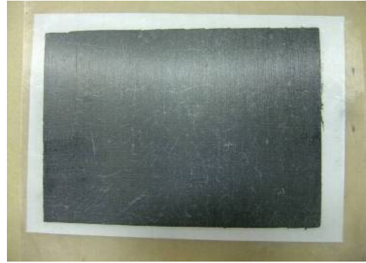
Figure 3. Completion of vibration plates of nano carbon tubes
