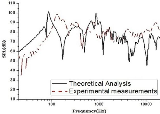
Figure 8. Verification of the experimental and analytic sound curves
