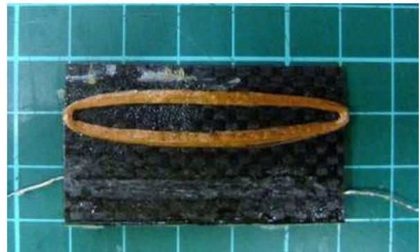
Figure 4 Completion of the exciter
