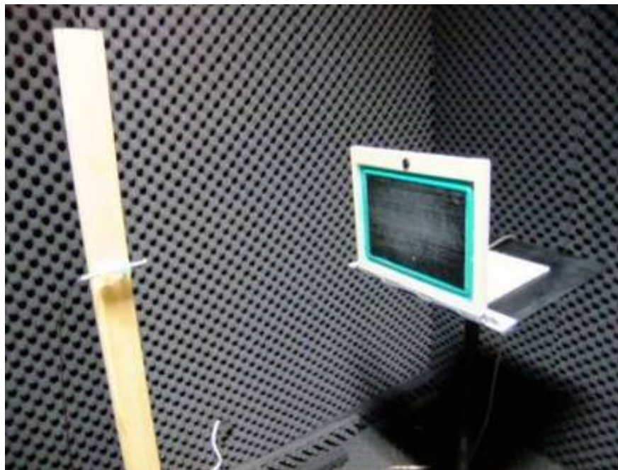
Figure 6. A illustration of the measurement of a planar loudspeaker
