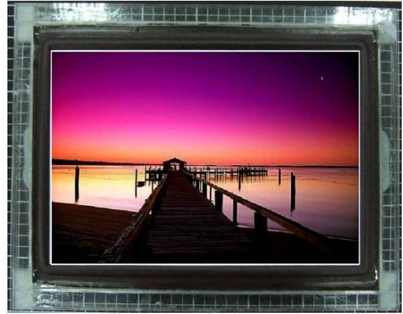
Figure 10. Application of planar loudspeakers with sandwich structure
