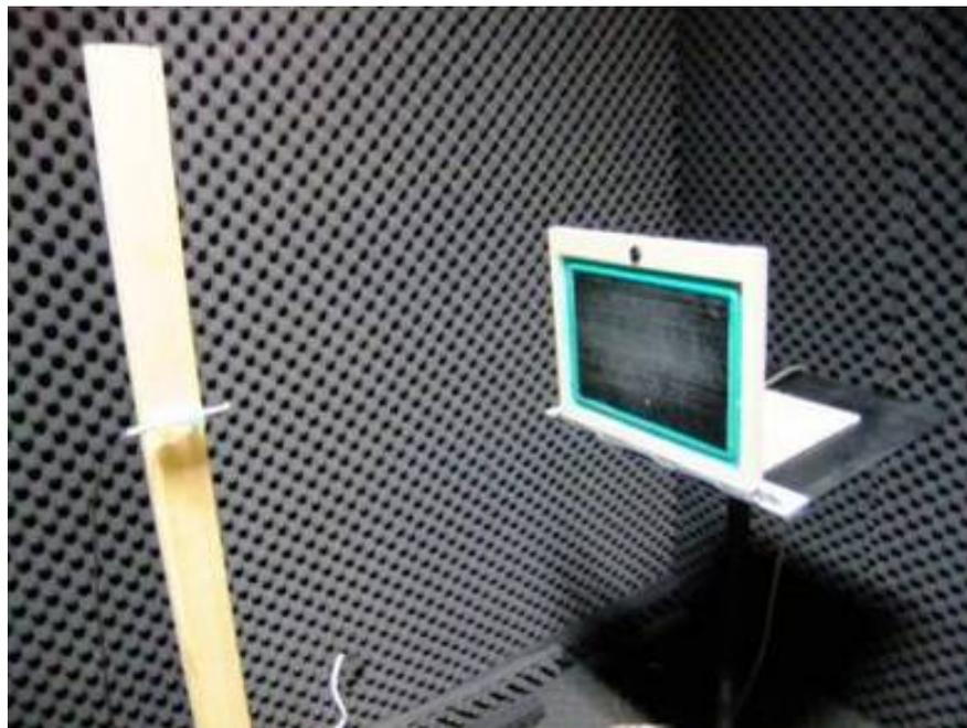
Figure 6. A illustration of the measurement of a planar loudspeaker
