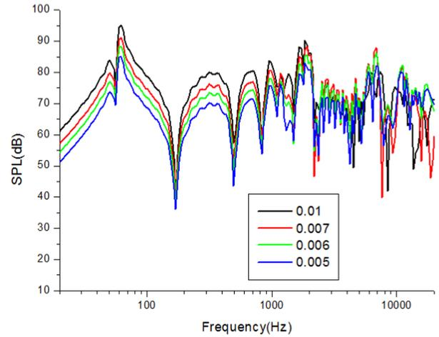
**Figure 7.** Sound pressure curve of mesh convergence
