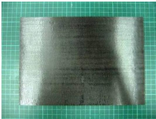
Figure 2. Completion of vibration plates of carbon fiber
