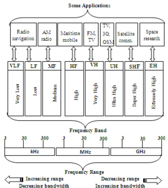
Figure 1. Radio Spectrum and some of its Applications (Adapted from [9])
