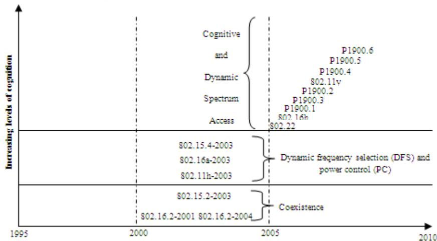
Figure 6. Evaluation of IEEE Standardization Activities from Coexistence to DFS/PC and finally to CR/DSA (Adapted from [43])
